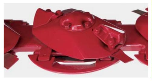
▲ Independent disc modules on the cutterbar make service and repair easy with bearings, gears and lubricant for each disc module individually sealed. Damage to one module does not spread to another. Ductile iron rock guards and easily accessible skid shoes will protect the cutterbed through many tough seasons.
