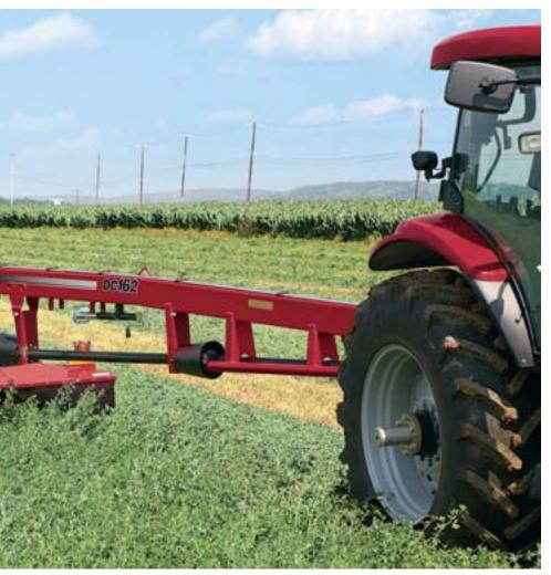
▲ Hydraulic header tilt lets you change cutting height on-the-go from the tractor seat. Use the maximum cutting angle for lodged crops or change to the minimum angle in rocky areas.
