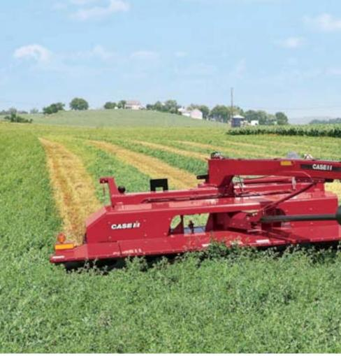
▲Torsion-bar conditioning roll pressure system allows conditioning rolls to automatically separate and clear slugs without stopping or lifting the machine.
