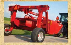
The high-clearance mainframe provides an exceptional header lift height of 20 inches for better clearance over headland windrows. The added height also allows the header to be easily carried over obstacles, ditches and waterways.
