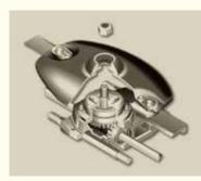
Standard knives feature a 12-degree pitch. For tough conditions like down crop, 18-degree knives are also available for more lift and a cleaner cut.
