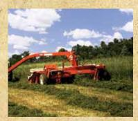
The Hesston® 1014 mower conditioner is introduced, the industry's first commercially available center-pivot mower conditioner.
