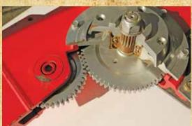
The internal spur gears offer high tooth-to-tooth contact at all times to transfer high torque and seamless power throughout the entire cutterbar.
