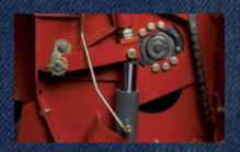
**Each cutterbar module** is driven by a segmented, reversible hex drive shaft for quick disassembly and reduced operating costs. The hex drive shaft is also designed to absorb the shock of hitting an obstruction, reducing the risk of damage.
