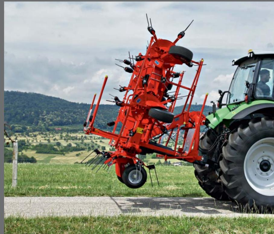
In spite of its considerable working width, the small-diameter rotors limit rear overhang so that it can be used with lower power tractors. The unique folding design allows for exceptionally low transport height and convenient operation from the tractor seat.
