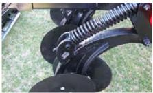
▲ Patented leveler features opposing blades on one common mount keeping the 870 shorter than competitors for better handling and performance in uneven terrain. Cast iron leveler arm provides added strength.
