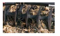
▲ Cushion Gang disk option features 26-in. (660-mm) blades on 12-in. (305-mm) centers. Narrower blade spacing provides better residue sizing.
