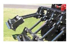
▲ The double-edged reel adjusts easily to suit the field conditions. The three settings for the reel are an adjustable down pressure mode, a float mode and pinned up.
