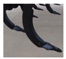
▲ Fracture root-limiting compaction and create good soil tilth with 2-or 7-in. (.05- or 2-m) tiger points®. Case IH tiger points perform a unique lift, twist and roll action that restores pore space and enables nutrient cycling in healthy soil.
