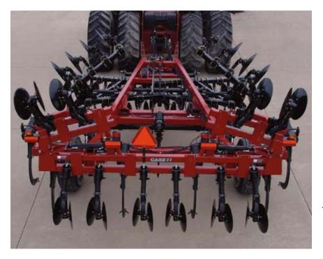
▼ Patented, double-edged reel components are much stronger than flats, shed wet soil, and resist over-penetration that plugs competitive reel designs.
