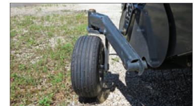
Pivoting pickup wheels for extreme conditions to ease wheel and tire stress
