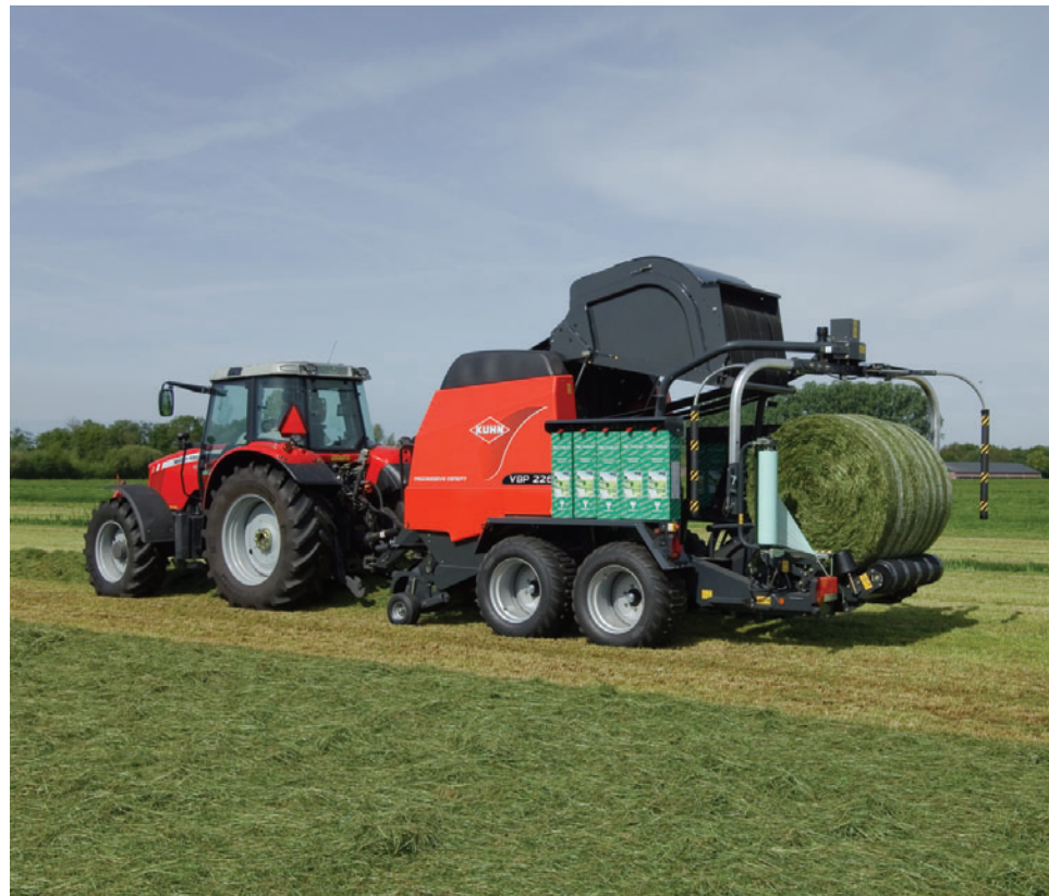
The bale is covered with 3 layers and 67% overlap
