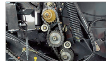
The second drive roller secures bale rotation even in difficult crops (standard on the VBP and optional on the VB)
