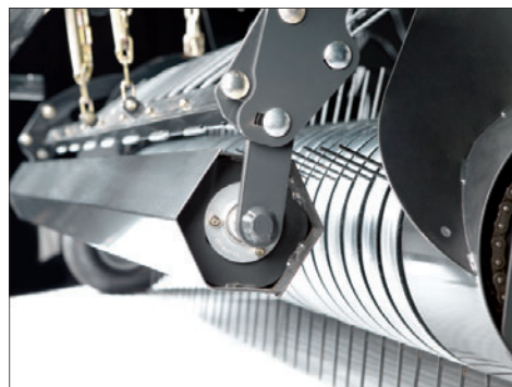
Low-profile, 5-tine bar pickup
